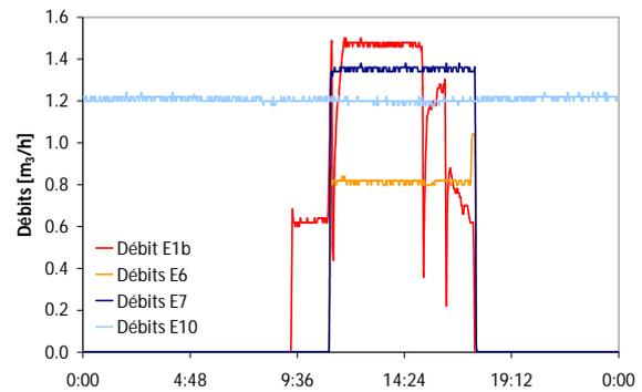
**FIGURE 6 - TYPICAL GRAPH (Q) OF A SOLAR AIR-CONDITIONING/HEATING SYSTEM IN AIR-CONDITIONING MODE, [15]**
