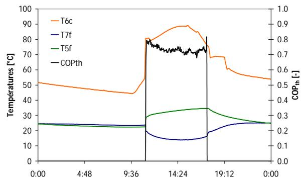
**FIGURE 8 – TYPICAL GRAPH (COP<sub>TH</sub>) OF A SOLAR AIR-CONDITIONING/HEATING SYSTEM IN AIR-CONDITIONING MODE, [15]**
