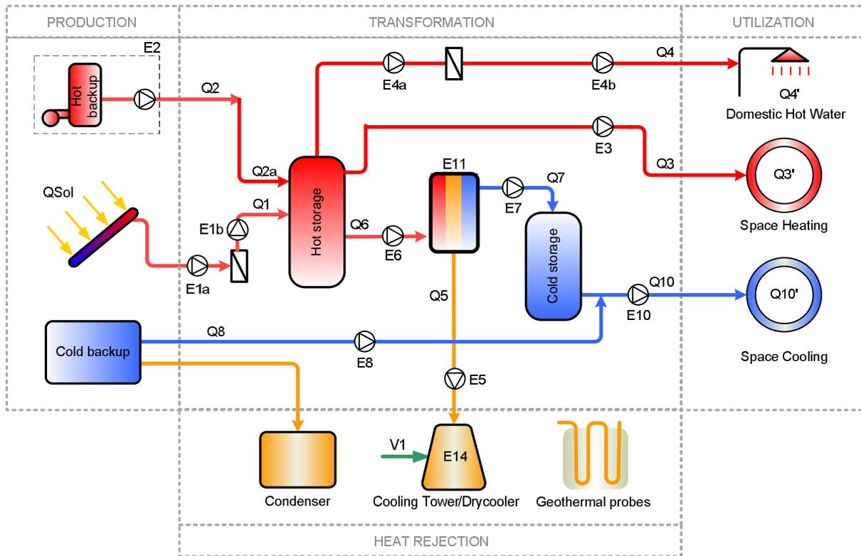
**FIGURE 4 - SCHEMATIC DIAGRAM OF A SMALL PRODUCTIZED SOLAR AIR-CONDITIONING/HEATING/DOMESTIC HOT WATER SYSTEM**
