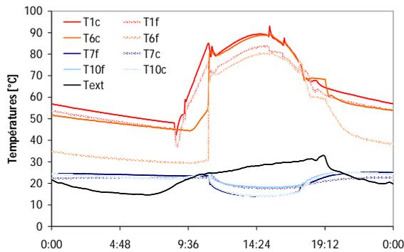
**FIGURE 5 – TYPICAL GRAPH (T) OF A SOLAR AIR-CONDITIONING/HEATING SYSTEM IN AIR-CONDITIONING MODE, [15]**
