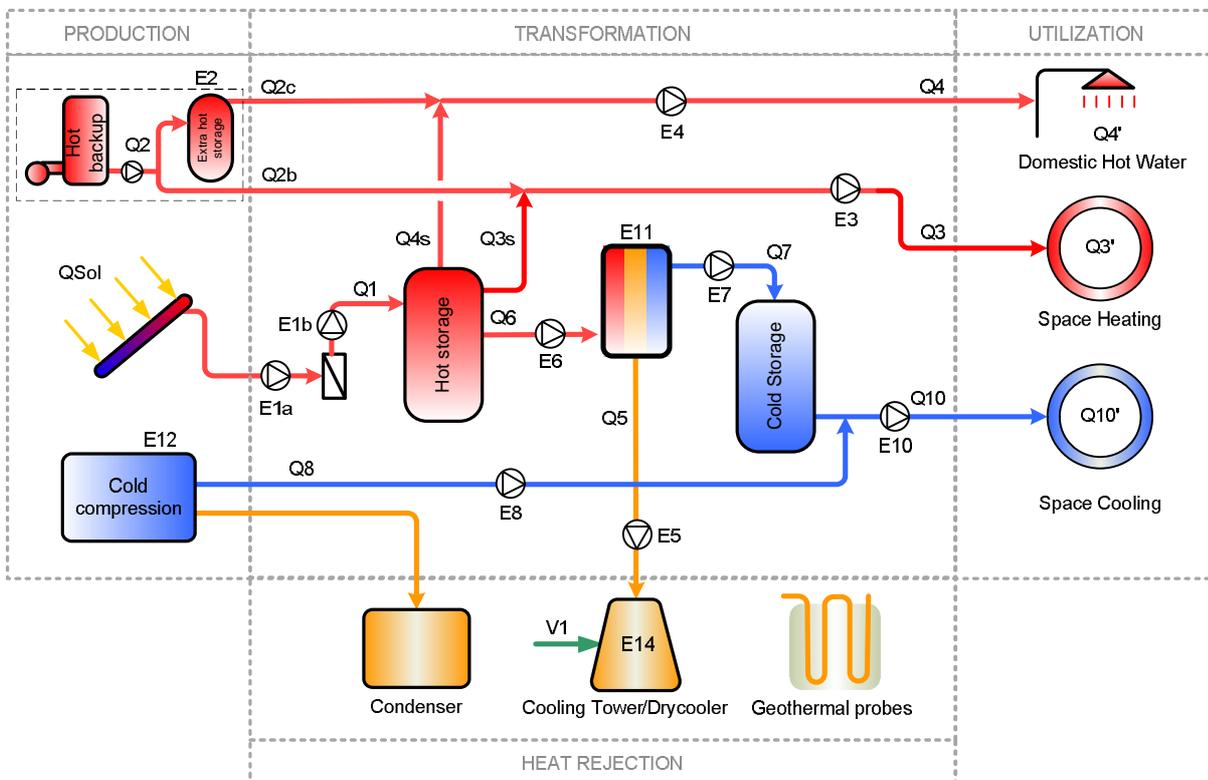
**FIGURE 3 – SCHEMATIC DIAGRAM OF A LARGE CUSTOMIZED SOLAR AIR-CONDITIONING/HEATING/DOMESTIC HOT WATER SYSTEM**
