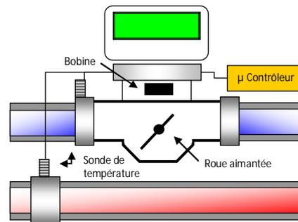
**DIAGRAM OF A THERMAL ENERGY METER**
