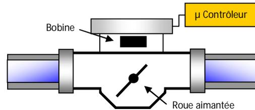
DIAGRAM OF AN IMPULSE METER
