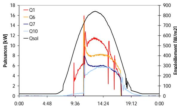
**FIGURE 7 – TYPICAL GRAPH (P) TYPE OF A SOLAR AIR-CONDITIONING/HEATING SYSTEM IN AIR-CONDITIONING MODE, [15]**
