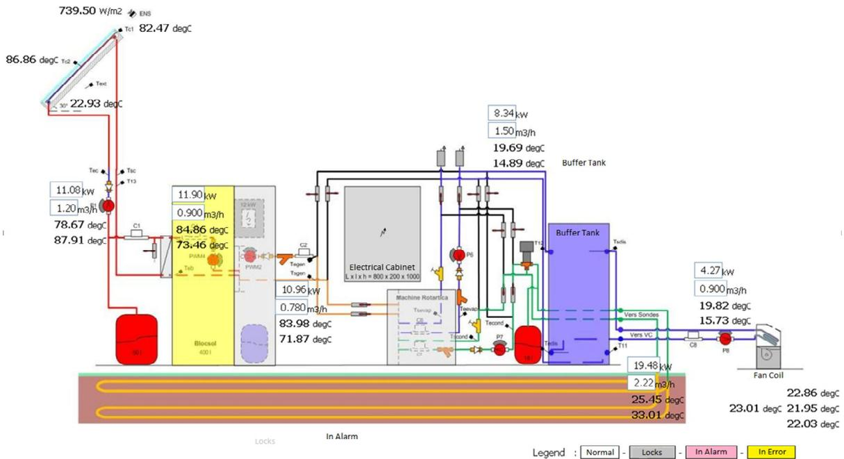
**FIGURE 9 – OVERVIEW OF HOW TO SUPERVISE A SOLAR AIR-CONDITIONING/HEATING SYSTEM FUNCTIONING IN AIR-CONDITIONING MODE [15]**
