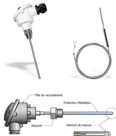
Temperature is usually measured using thermistances whose resistance decreases as temperature increases (Pt100 or Pt1000 platinum probes). They transmit an electrical signal proportional to the temperature. Standard NF EN 60751 defines two classes of accuracy (A and B) for temperature probes.
