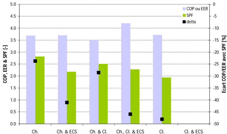
**FIGURE 11 - COMPARISON OF COP AND EER WITH SPF BASED ON MONITORING DATA ON LOCATION DEPENDING ON SYSTEM CONFIGURATIONS [28 TO 36]**
