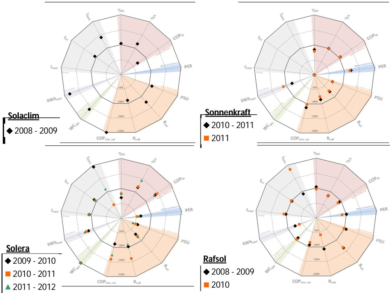
**FIGURE 10 – ILLUSTRATION OF OVERALL SYSTEM PERFORMANCE OF A SOLAR HEATING/AIR-CONDITIONING/ DOMESTIC HOT WATER PRODUCTION SYSTEM (SOLERA [27], SOLACILM [24], RAFSOL [25] & SONNENKRAFT [26] SYSTEMS)**
